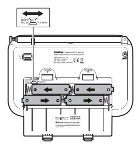
1. Open the battery cover on the rear of the unit by pushing the latch downward.
