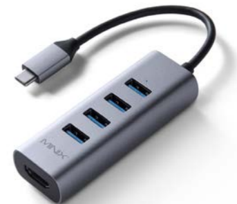
NEO C-UH Aluminium USB-C to 4-Port USB 3.0 And 4k @ 30hz HDMI Adapter.
